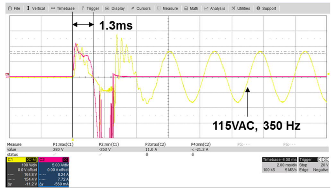
Figure 11 115V 350Hz AC applied to activate the fuse integrated in DEI1604. It was arced to open at 1.3ms
